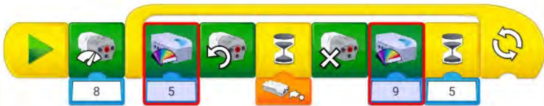
Change the color of the hub is easy to use to understand what part of the program is currently running on the robot.
